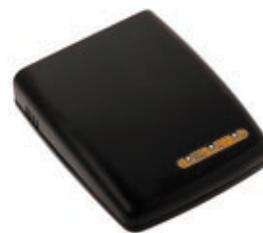
The SmartLiving system can be remote controlled and programmed over the PSTN line through a SmartModem. The SmartModem must be connected to a computer which runs INIM's SmartLeague software. The modem interfaces with the computer through a USB port. It is powered directly through the USB port thus avoiding the need of any external power supply. Its reduced size makes placement unproblematic.
