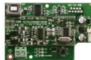
The SmartModem200 modem board allows you to programme and control SmartLiving series systems using a standard dial-up modem protocol. The SmartModem200 is an add-on board which connects to the SmartLiving serial port. It is capable of reaching a data transfer rate of 57600bps and so greatly reduces remote programming times. The SmartLeague software programme allows you to choose to work on the SmartLiving system through the modem-on-motherboard or via the SmartModem200 board.
